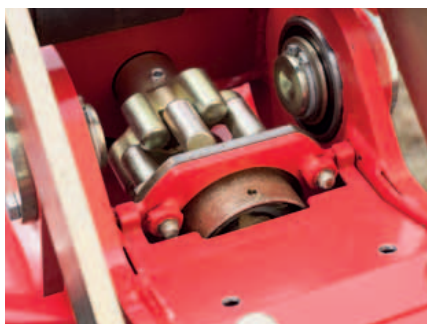
Kverneland HexaLink finger clutch permits a 180° folding of the rotors for transport.
