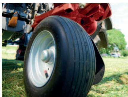
Kverneland 8576 can be equipped with a third wheel to ensure correct set-up of the tedder independent from tractor and driver.
