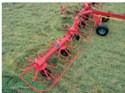
For border tedding the 3 outer rotors are pivoted, to secure evenly inward spreading.
