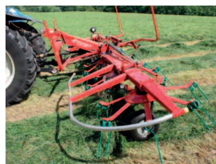
New aluminium rail guards, which are low in weight, but still extremely impact resistant.
