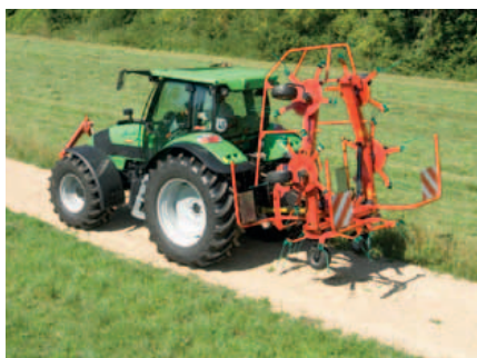
Kverneland Taarup 8460 folds hydraulically from working to transport position and vice versa.
