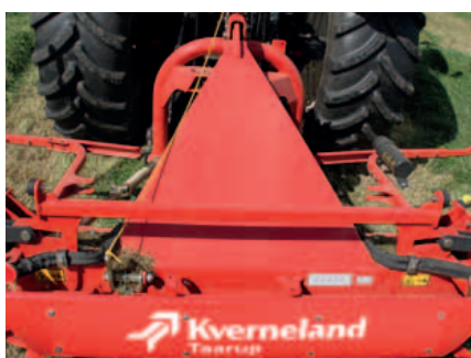
Strong and sturdy mainframe design with V-shaped central unit.
