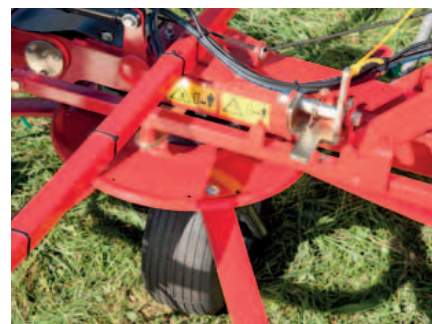
Kverneland Taarup 8446 and 8452 are centrally adjusted for border tending.
