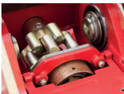
Kverneland Taarup HexaLink finger clutch permits the rotors to fold 180° for transport.
