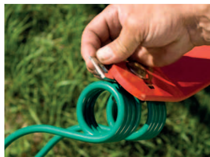
Easy and simple adjustment of tine angle.
