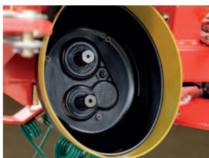
With the optional reduction gearbox it is possible to place night swaths.
