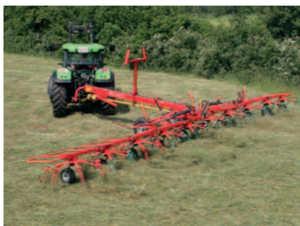
80° turning angle ensures excellent manoeuvrability.
