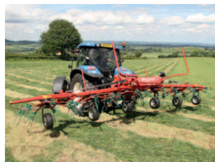
Kverneland 8576 can be equipped with the optional hydraulic headland kit.
