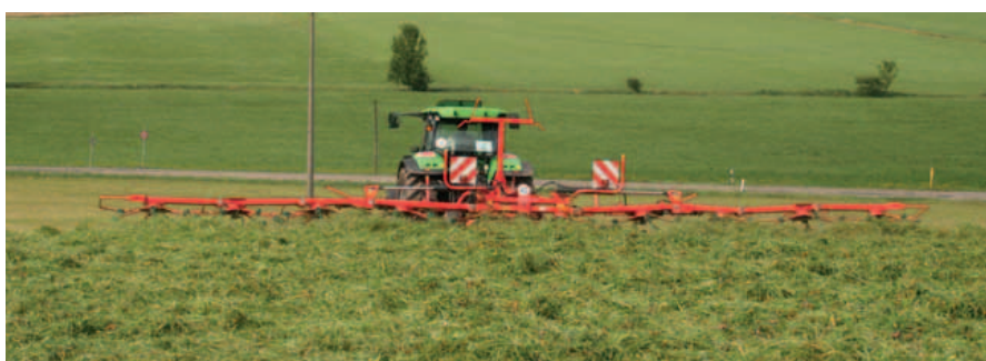
The hydraulic suspension supports protecting the ground under all conditions. Three working modes of the suspension can be chosen.
